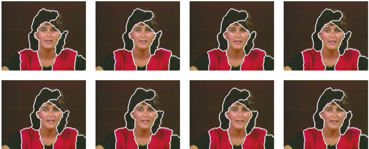
Fig 15. Segmentation results on the “Miss America” sequence. Sample frames are chosen where the only major objection movement occurs in the sequence. Frame 74-83. The first 150 frames are segmented as a group and the minimum object duration is 15 frames or 0.5 s. Frame size 176 x 144.
