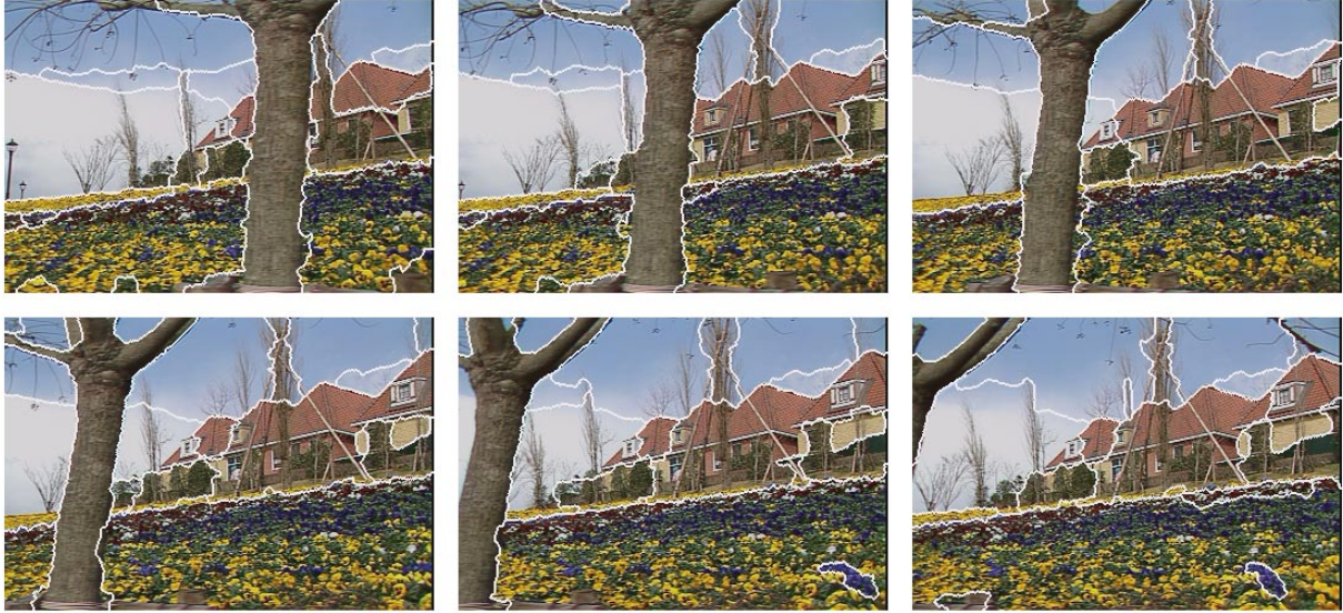
Fig 16. Segmentation results on the “flower garden” sequence. Sample frames are chosen: frame 1, 11, 21, 31, 41, and 51. The first 60 frames are segmented as a group and the minimum object duration is 3 frames or 0.1 s. Frame size 352 x 240.
