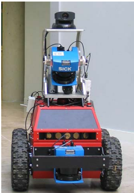
Figure 1. The research platform. At the top is a pan-tilt camera. In the middle is a laser scanner mounted on a mechanical oscillator that allows a 2D laser scanner to capture 3D scans of the environment. At the bottom is a fixed laser scanner which is used to obtain 2D scans parallel to the ground plane.
