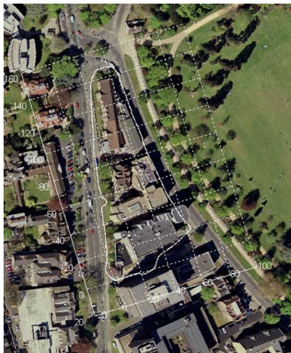
Figure 17. An aerial image of the workspace with the final estimated vehicle trajectory and metric grid superimposed upon it.
