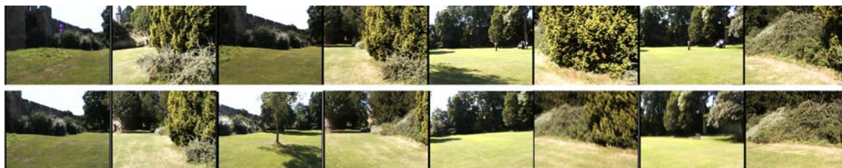
Figure 24. Two matching sequences of images ( \mathcal{A}, \mathcal{B} ). These images correspond to the bottom right loop closure in Fig. 25(b). It is not immediately apparent that this is indeed a loop-closure. In the third column along the sequence, the two images look very different due to a substantial difference in viewpoint.
