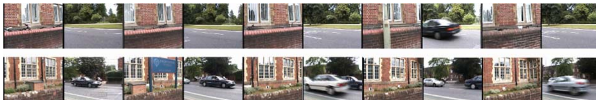
Figure 7. An erroneous loop closure detection in the presence of ambiguity. This is one of the sequence matches that results by applying the sequence detection algorithm directly to the matrix in Fig. 6. Although the two sequences are indeed similar, repeating visual entities such as wall patterns, window styles, vegetation, results in a Type I (false positive) error.
